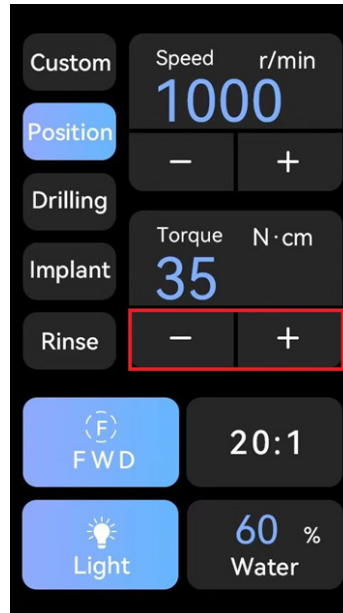
Fig. 10 Adjusting the upper limit of torque
