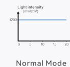
Constant light intensity: 1000-1200mw/cm<sup>2</sup> Suitable for most treatment scenarios, such as fillings, restorations, etc. Time setting: 5s, 10s, 15s, 20s
